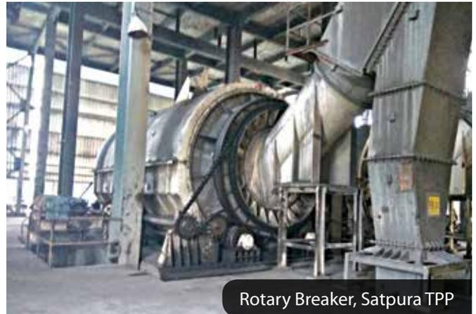
Rotary Breaker, Satpura TPP
