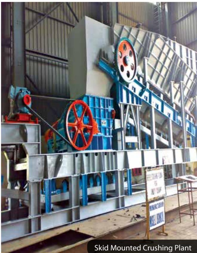
Skid Mounted Crushing Plant
